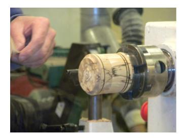
You can then finish the top, by taping the joint tightly to hold the work together, and using very gentle smooth cuts, and then finish the bottom by reverse chucking. (Tip – use a straight edge to ensure the bottom is slightly concave so it will sit flat.) Thanks Phil, for an informative and enjoyable session. (Phil's handout is included below.)
