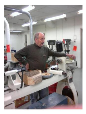
Phil used a screw chuck to initially mount the piece, then showed how he forms the outside rough shape and makes a tenon to reverse the mounting. He advises that a larger diameter tenon provides better support. The length of the tenon should be less than the depth of the jaws so that the top of the
