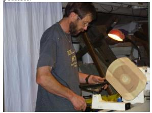
A second demo showed us how Peter can hollow out the inside of a form without any apparent opening for the tool to enter. This is basically a process of carefully removing a "plug", doing the hollowing cuts, and then replacing the plug with precise grain alignment so it blends back in and is virtually impossible to find.
