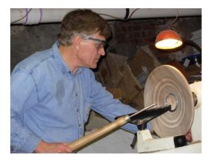
He provided an overview of his cutting style, which uses a 45 degree angle on both tool and body language. He emphasized the critical use of spigot cut and chuck application, demonstrating how to gauge both with the protractor.
