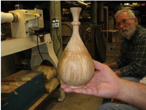
These pieces begin with a tenon formed on each end, which are eventually parted off and used to remount the hollowed form and construct an insert to plug the bottom hole.
