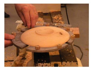
And then cuts it in half on the band saw. He pointed out that the mating surfaces on the outer rim must be sanded perfectly flat or they won't meet properly.
