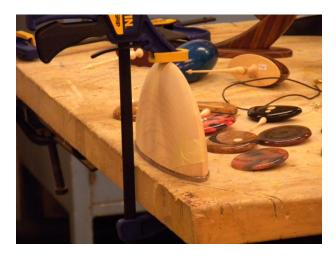
For aesthetic purposes he recommends using wood that is consistent in color. The base is made by tilting the band saw base at an angle, but be sure to keep it wide enough at the top to support the 1/8" hole for the brass mounting pin.
