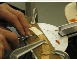
In addition to Noden's patented Inlay Razor system, Geoffrey also recommended a few accessories to help with accuracy and efficiency. His router used to cut the channels and trim the arcs for the inlaid tiles was a small Bosch Colt router. Noden used a plunge base and fence system sold through MicroFence, Inc. (http://microfence.com/plunge-base-c-22.html) The base allowed precise depth cutting and the circle cutting guide allowed for repetitive cutting of the inner and outer arcs.
