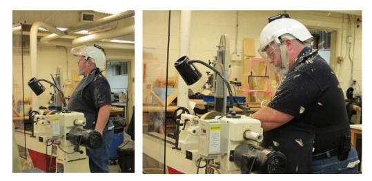
Grumbine began his turning demo by mounting a prepared blank of green maple and cut a narrow vee groove in the spud for mounting in a set of high profile jaws mounted in his chuck.
