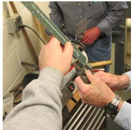
Don's demonstration included the use of some commercial tool positioning jigs and devices as well as the Raptor angle finders for doing jig set-up and measurement. Members were invited to bring in a tool to be sharpened and Don went through the steps for setting up each sharpening situation.
