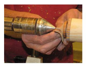
Rosand does is final sizing on his acorn bird houses with a nifty little side-scraper. Gently tilting the tool gives an ever-so slight scrape against the edge of the stub tenon and allows for accurate fit-ups. Final sanding of the tops is done by flipping the cone 180 degrees and gently holding things in place with the tailstock. Rosand even goes as far as to use some tiny scraps of ebony to turn the miniscule perch for his bird houses. All of his pieces were finished with a
