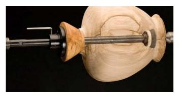
Robert Jay shared a special mandrel made by Kelton Industries for hollow form turning. One end fits into the lathe's #2 Morse socket and the other end supports a screw-in sanding pad. This product is available through Craft Supplies.
