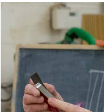
then honing the skew spanning the hollow grind area
