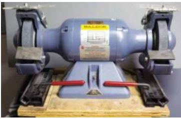
left rest set at 45 degrees, right set just below 90 degrees
