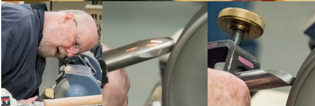
The Ellsworth Signature Gouge requires a special jig which rotates the tool properly on the wheel. Freehand is also an option, but the movement takes practice.
