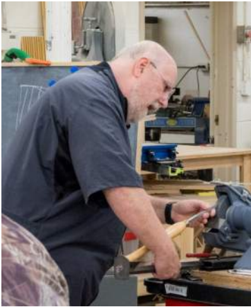
sharpening skews on the left hand rest
