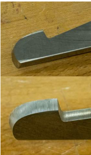
scraper edges at less than 90 degrees
