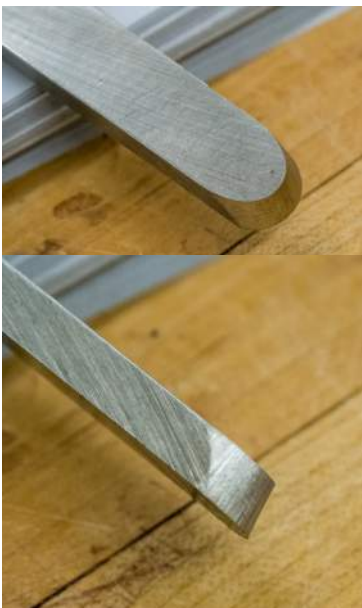
scraper cut with the 45 degree platform rest
