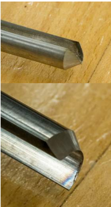
gouge cut with the 45 degree platform rest
